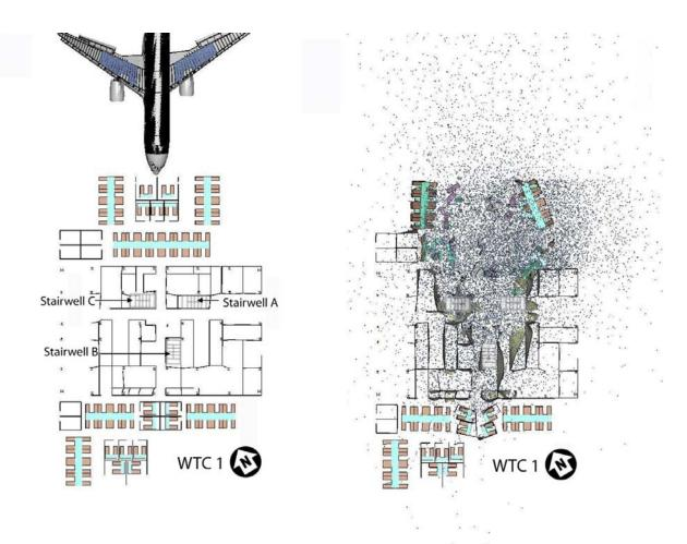
Figure 5–2. Computer simulated impact damage to WTC 1 on floor 95 at 0.7 s after impact with stairwells superimposed.
