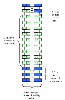
Figure D-3. 44 in stair configuration in building EXODUS.
