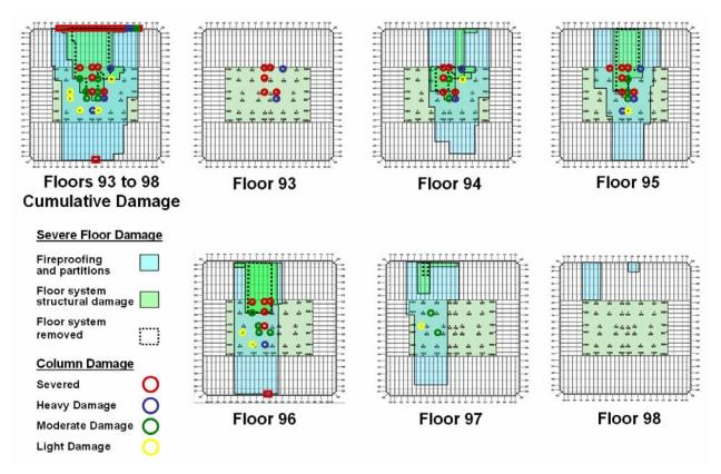
Figure 5-3. Calculated damage to floors 93 through 98 in WTC 1.
