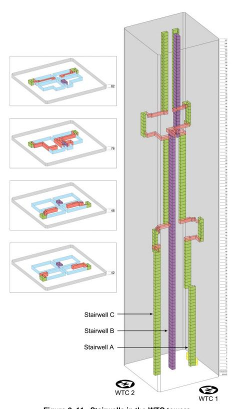
Figure 2–11. Stairwells in the WTC towers.
