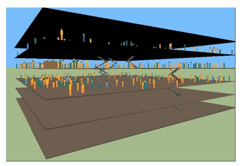
Figure D-1. 3-D view of a phased evacuation showing floors 45 – 50 (Exodus).
