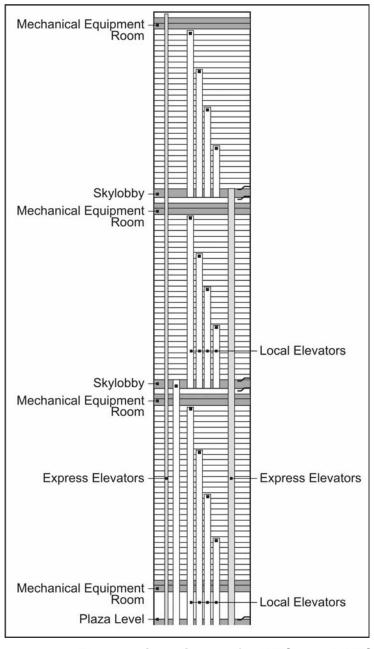
Figure 2-14. Elevator riser diagram for WTC 1 and WTC 2.
