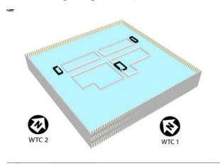
Floor 76 Stairs A, B, and C transferred, with Stairwells A and C moved outside the core.
