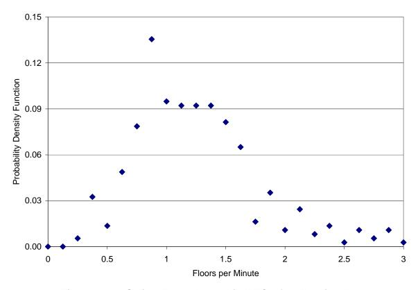
Figure 10-4. Stairwell travel speed in WTC 1 for all stairwells.
