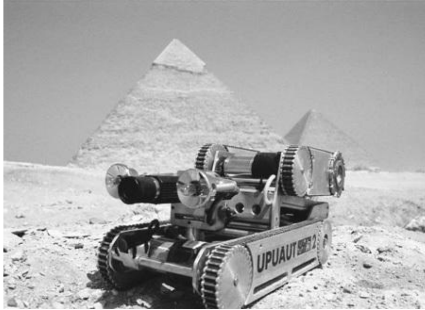
Figure 1.11. Gantenbrink's robot, Upuaut II, which was used to explore the shafts in the Great Pyramid in March 1993
